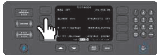
Figure 19: Test Mode: Blower Test
