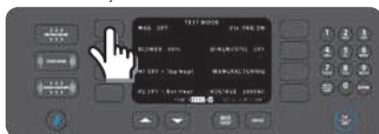
Figure 17: Test Mode: Magnetron Test
