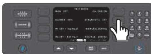
Figure 24: Test Mode: Diagnostic Mode On/Off
