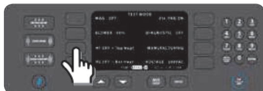
Figure 21: Test Mode: Top Heater Test
