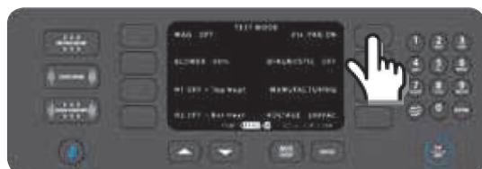
Figure 23: Test Mode: EC Fan Test
