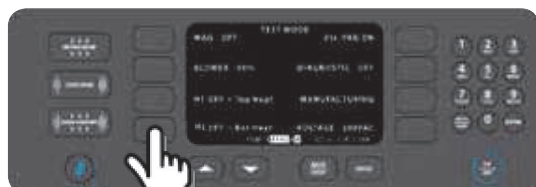
Figure 22: Test Mode: Bottom Heater Test
