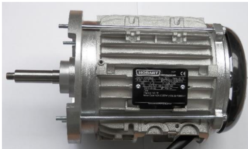
Photograph 5. Externally cooled cast aluminium motor.
