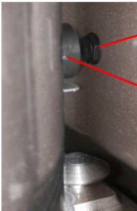
Photographs 6 & 7. HSM30 and HSM40 bowl magnet and interlock switch.
