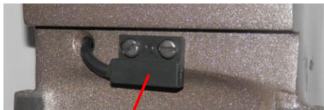
Bowl interlock switch (situated behind the upper splash shield).
