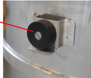
Photographs 6 & 7. HSM30 and HSM40 bowl magnet and interlock switch.
